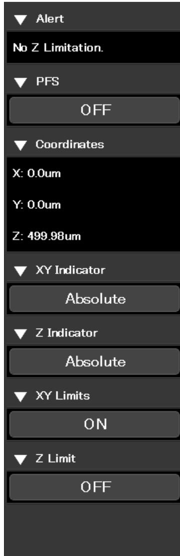
This subscreen allows the user to set the XY software limits.
