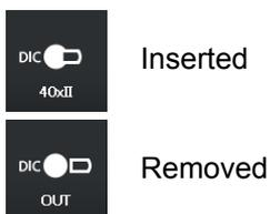
Indicates the DIC analyzer slider in/out status.
