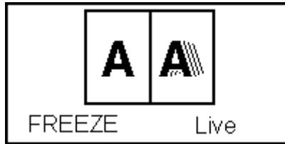
You can split the screen into left and right halves and display a still image in the left half and a live image in the right half for image comparison.
