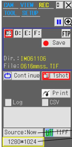
The CCD source setting represents the CCD mode during image acquisition when you freeze, save, or print images.
