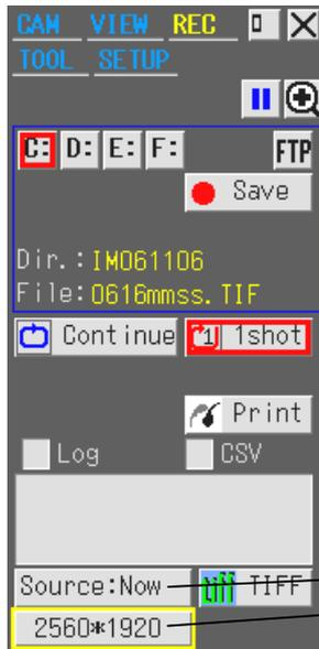
“CCD source setting” represents the CCD mode during image acquisition when you freeze, save, or print images.
