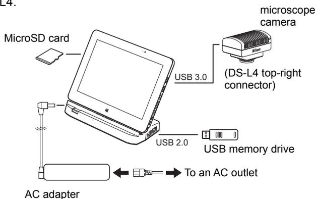
Note: The microscope camera must be connected to the USB 3.0 connector. The USB 3.0 connector is at the top-right of the DS-L4.
