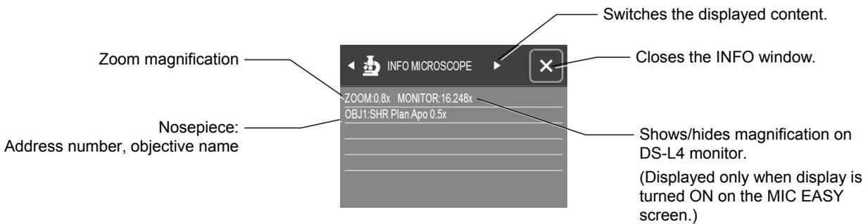
In this chapter, you configure the information on the optical elements attached to the microscope. The information of the optical elements you entered here is displayed on the DS-L4 screen.
