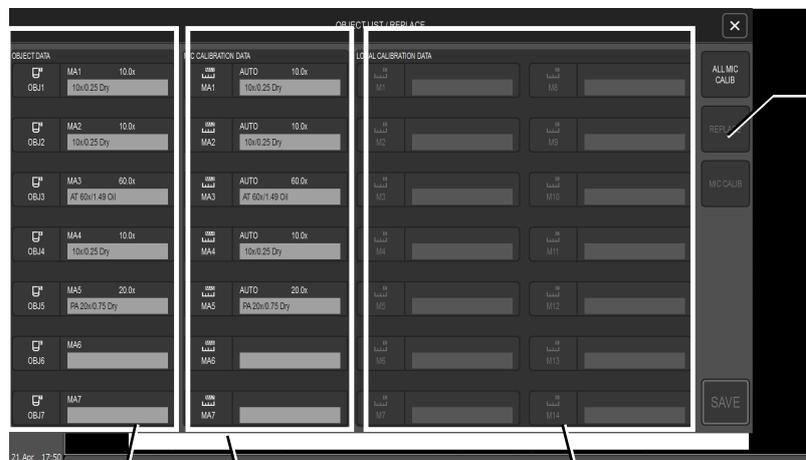
Select an objective address and local calibration setting number, and then tap [REPLACE].
