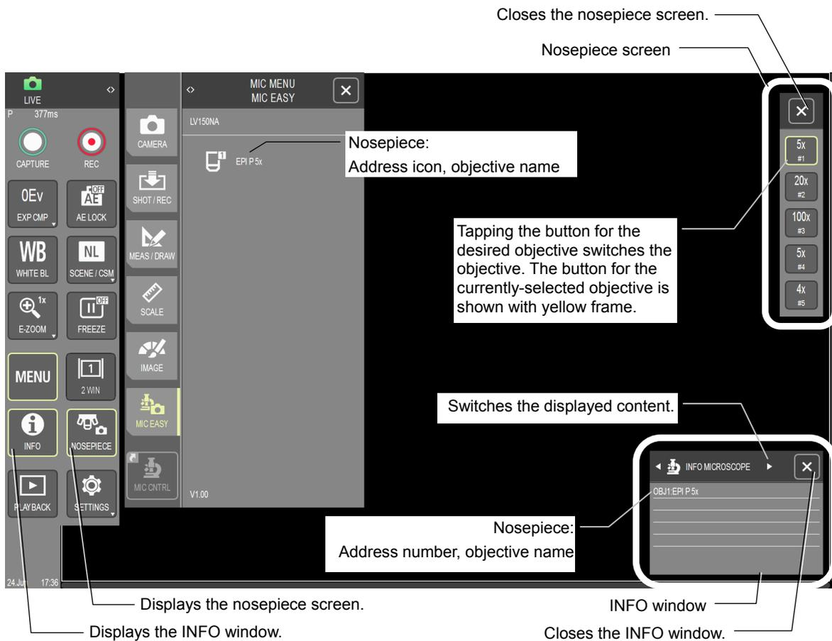
Viewing the Status of Microscope on DS-L4
