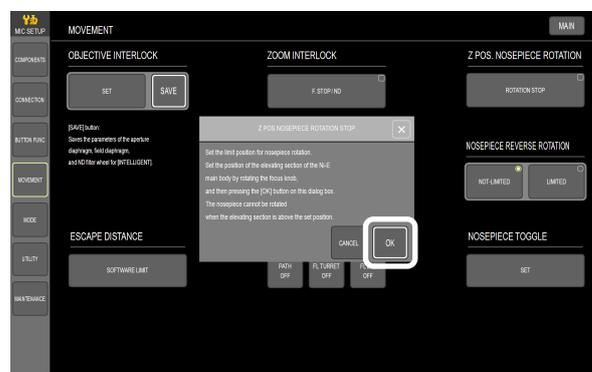
Since the focal depth of the objective with low magnification is deep, such an objective may be positioned close to the specimen when used. When the objective is switched to the high magnification objective in this situation, the tip of the objective may contact with the specimen. In order to prevent this, you can prohibit rotation from address 1 to the next address 6 (for sextuple nosepiece) or from address 1 to the next address 7 (for septuple nosepiece) with this setting.
